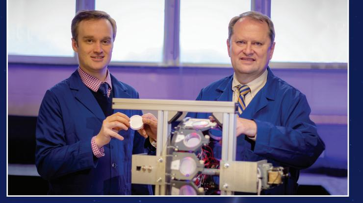
HERE ON EARTH Kiss and his colleagues have been involved in nine NASA space shuttle missions and five NASA-contracted SpaceX missions. Above, postdoctoral researcher Josh Vandenbrink and Kiss (l-r) load samples onto a clinostat, a device that simulates microgravity and helps them analyze results from spaceflight experiments.
