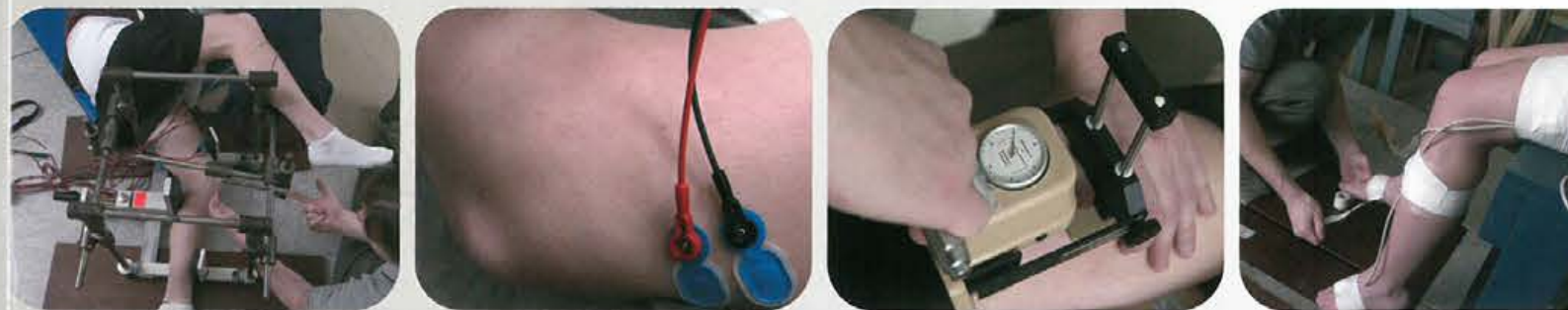
Dr. Sandy Shultz uses a variety of devices to learn more about the strategies that will prevent an ACL tear. Pictured above are a Reflex Testing Apparatus created by Shultz, a close up of sensors attached to the knee, another instrument called the KT 2000 Knee Arthrometer and a researcher taping sensors onto a volunteer.
